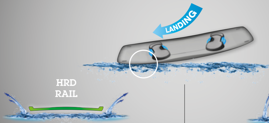
HRD RAIL Rail shape deflects the water away. The board slides over the water when landing.
