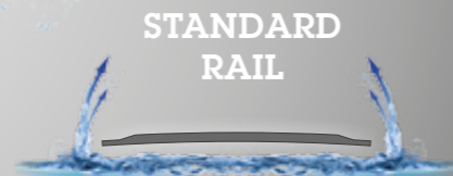
STANDARD RAIL Rail shape runs through the water. The board grips into the water.
